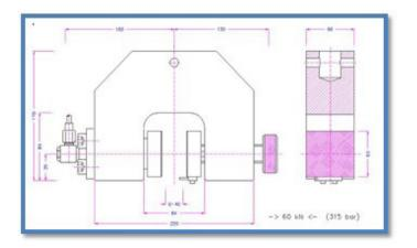
A Hydraulic grips with single actuator, single actuator grips have one side adjusted by manual tightening action screw, and the grips are suitable for offset sample alignment for shear test-ing
