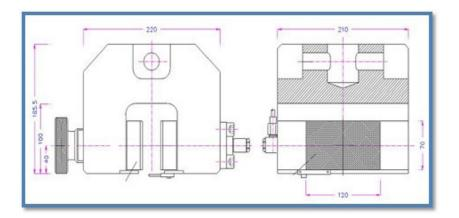
A Hydraulic grips with dual actuator; ideal for all types of samples, rubber, plastic dumbbells, metal, fabrics and composites (depends on rating).
